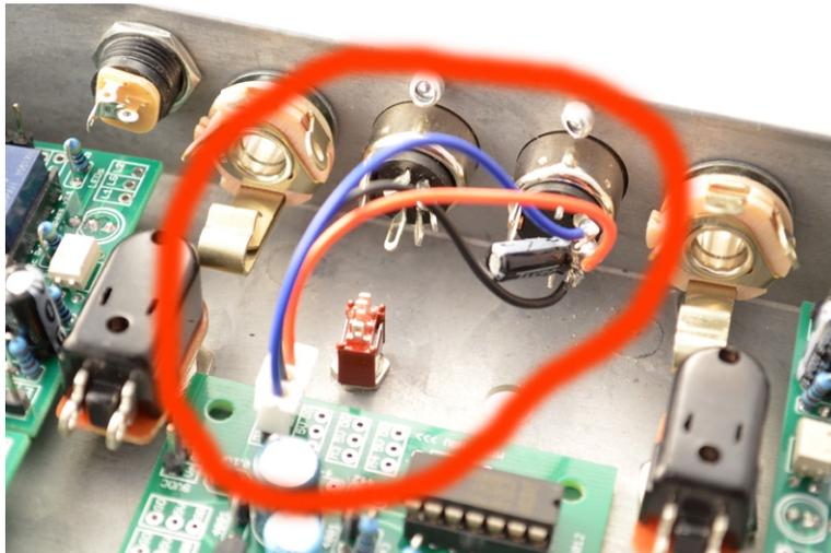
Cut and trim the leads on 2-pin wired header connectors as follows:
