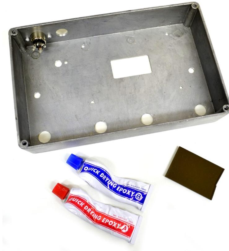
Wipe off the inside of the enclosure, then remove the paper backing from both sides of the lens and set it carefully aside.
