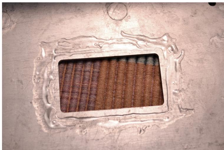
Carefully place the lens over the opening - **YOU ONLY GET ONE CHANCE** - so take your time and line it up before allowing it to contact the epoxy!!!
