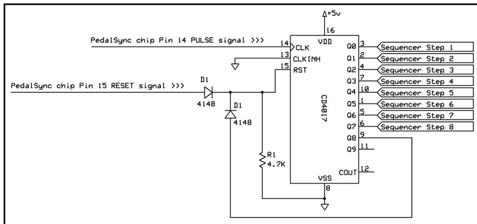
When sending a Pulse/Reset connection out of an enclosure, consider a TRS jack with PULSE at the Tip, RESET at the Ring, and Ground at the Shield.
