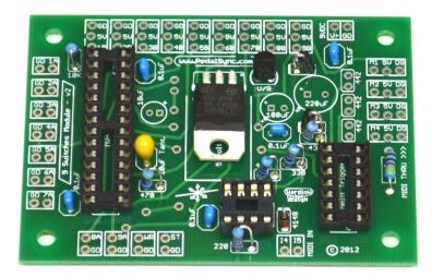
Solder the 3 electrolytic capacitors in place. The value and polarity are indicated on the PCB - the square hole is +, and corresponds to the longer lead on the cap.
