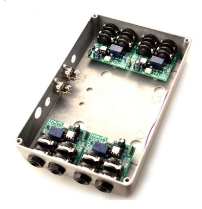
The audio from each module needs to be connected to the adjacent module. Connections for Audio Input and Output are on both sides of each module. Use a solid jumper wire to make the connection. The wire can be a leftover lead from a component.
