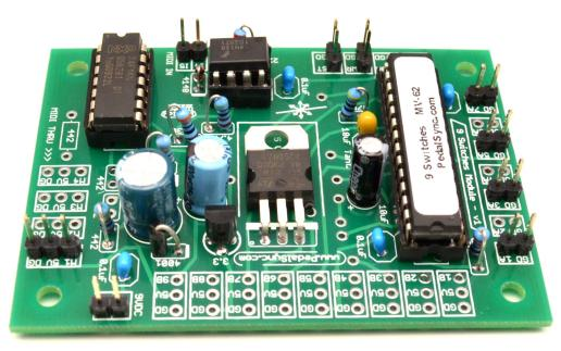
Attach the 2-pin headers to the 1, 3, 5, and 7 switch inputs, the 9VDC power input, the MIDI IN, the WR/GD- write switch input, and the ST/GD - status LED output.
