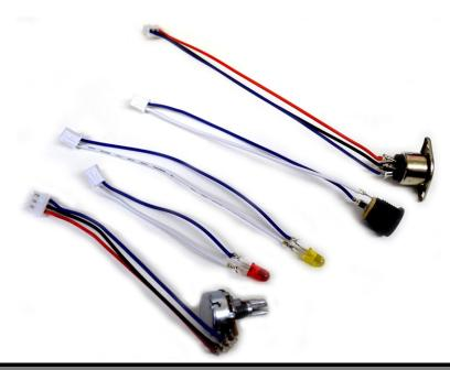
Cut and trim the leads on a 2-pin connector to 4.5 inches, then cut and bend the legs to the Tempo LED and solder in place.
